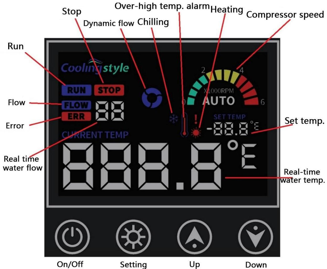
The display screen is divided into a display area and an operation area, as shown in the figure above.
